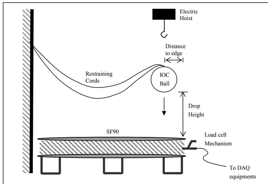
Figure 2.4 Test Setup
