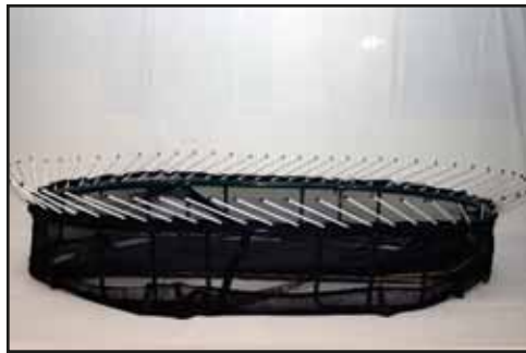
Figure 9: The rest of the rods inserted through the enclosure holes and into the frame sockets
