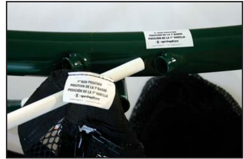
Figure 7-A: Placing the first rod
